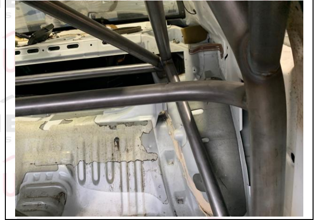
PHOTO 13 SHOULDER HARNESS ATTACHMENT - CO DRIVER
