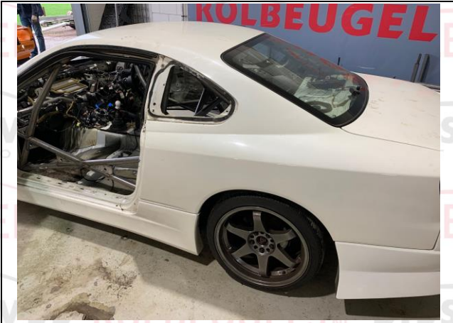
PHOTO 10 ANTI-INTRUSION DOORBAR - DRIVER
